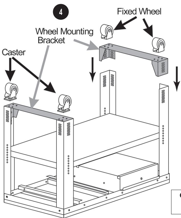
Attach the two wheel mounting brackets in the manner shown in Fig.4, using the M6 nuts bolts and lock washers supplied.
