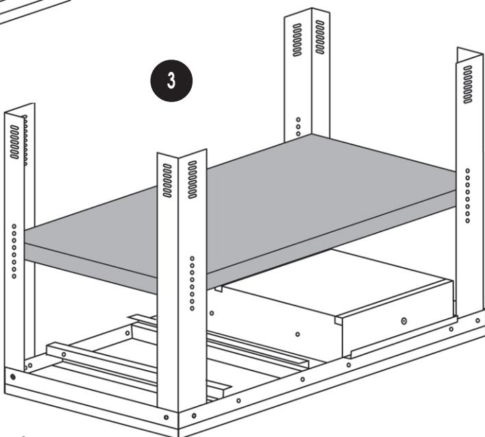
Attach the shelf in the manner shown in Fig.3, using the M6 nuts bolts, lock washers and flat washers (supplied).
