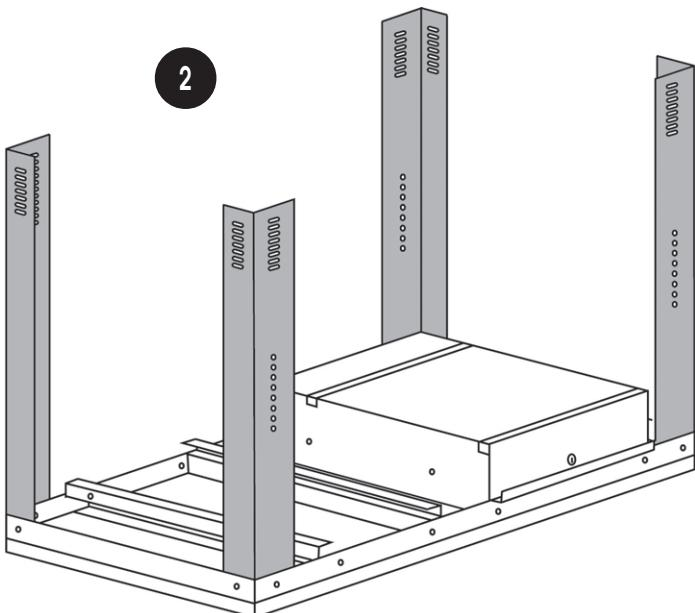
Attach the legs in the manner shown in Fig.2, using two M6 nuts bolts, lock washers and flat washers (supplied), per leg.
